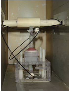
The actual cell perfusion apparatus used for experiments.
