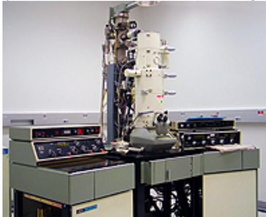
**The OSEL's** electron microscope gains extra protection against image-blurring vibrations because beneath the assembly is a concrete "island" flush with but not abutting the surrounding floor, supported by heavy-duty isolation mounts supplied by Kinetic Systems.
