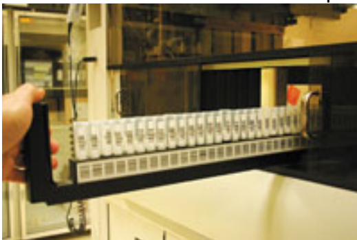
Loading sample racks into the Abbott Prism system
