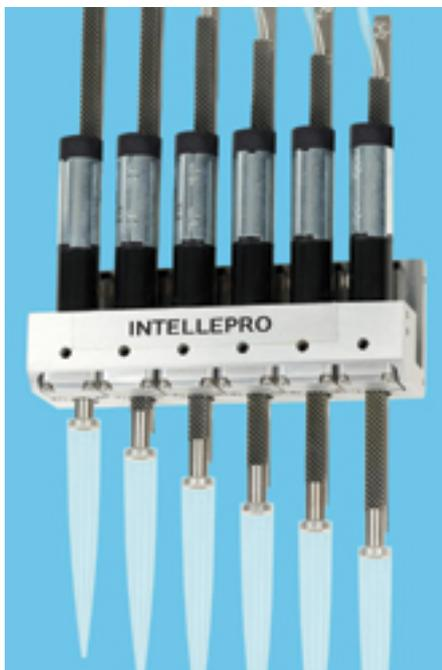
There is more to compactness than just using smaller motors. IntellePro Inc. faced a serious challenge when the company needed a system that would accommodate pipettes on 18 mm centers that would also be capable of driving six probes independently with up to 125 mm strokes. IntellePro worked closely with a biotech integrator (Protodyne) in both the design and development of the pipette automation system to ensure the performance and life expectancy required by Protodyne's "Radius" line.
