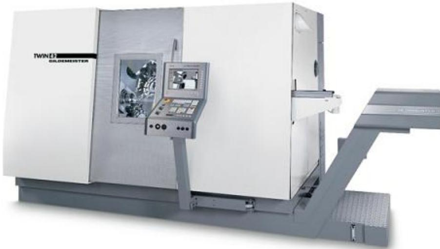
This machine joins multiple DMG TWIN 65 and TWIN 42 machining centers, each with an upper B-axis to complement the Y-axis and driven tools and create the contours and sophisticated geometries needed at Stryker. These turning machines have the Siemens Sinumerik 840D onboard, which enables precise and transferable control of spindle and axis movement variations via compile cycles, so Stryker Experimental engineers can make more rapid changes in their production scheduling, according to this user.
