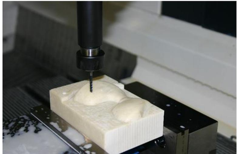
aesthetic feedback by surgeons, though not for formal trials or surgical use. As a result, Stryker maintains a variety of machine tools and other metalworking equipment at its Kalamazoo facility. Basic milling and drilling equipment is here, alongside three- and five-axis CNC machining centers and EDMs.
