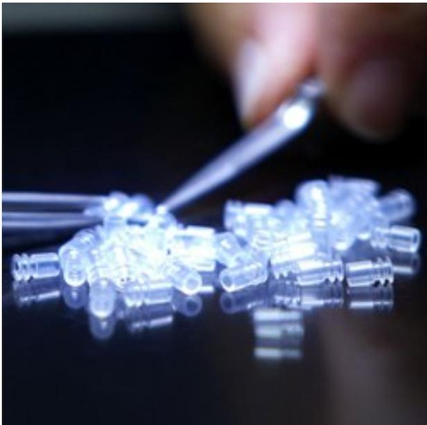
**These seals for pacemakers have been injection molded in liquid silicone.**
