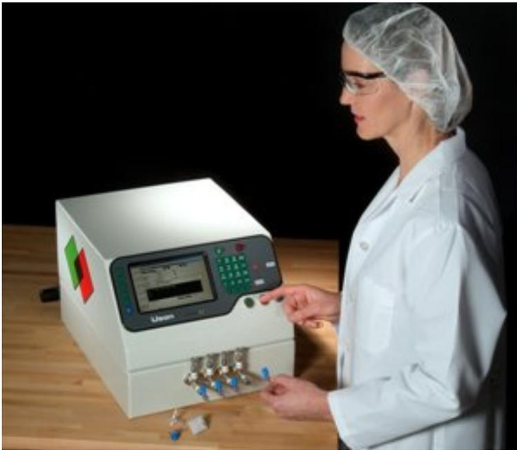
**USON's multichannel VECTOR Leak Tester, here being used to leak test check valves, can be configured with up to 10 independent test channels and I/O capability up to 72/122 different programmable steps.**
