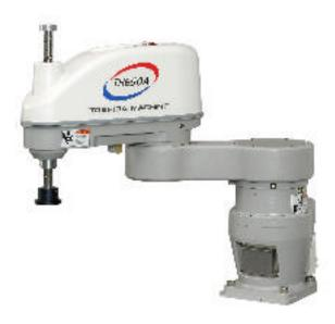
An industry first for SCARA robots, Toshiba Machine's TH-A Series is equipped with highly rigid gears for each axis. Proven successful in 6-axis robots, these gears provide quicker acceleration/deceleration, a longer life span, and easier maintenance.
