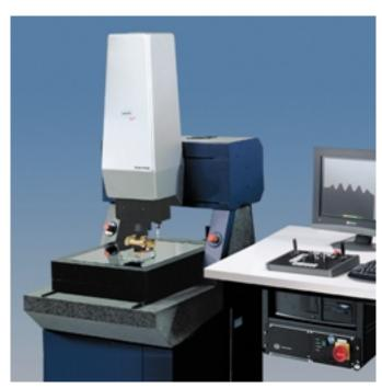
This is the concept for Werth Messtechnik GMBH's introduction of the fixed-bridge models of the ScopeCheck device. Solid base granite frames with mechanical guides offer economical solutions. Dirt-resistant guides and scales allow operation under the roughest of production conditions. Precision-guided measurement axes are isolated from each other. Measurement range of this series is up to 3,500 mm in the X-axis, and 1,750 mm in the Y-axis.
