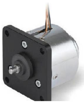
Johnson Electric introduces the Saia ULE Series Linear Stepper Motors. Available in unipolar or bipolar configurations, these motors provide constant positioning force to 400 N over full travel lengths to 300 mm in ambient temperatures ranging from -15 to  $60^{\circ}$ C. Their compact 55 x 55 mm design envelope and NEMA 23 mounting flange enables the ULE series to be mounted in space-restricted applications with great flexibility.
