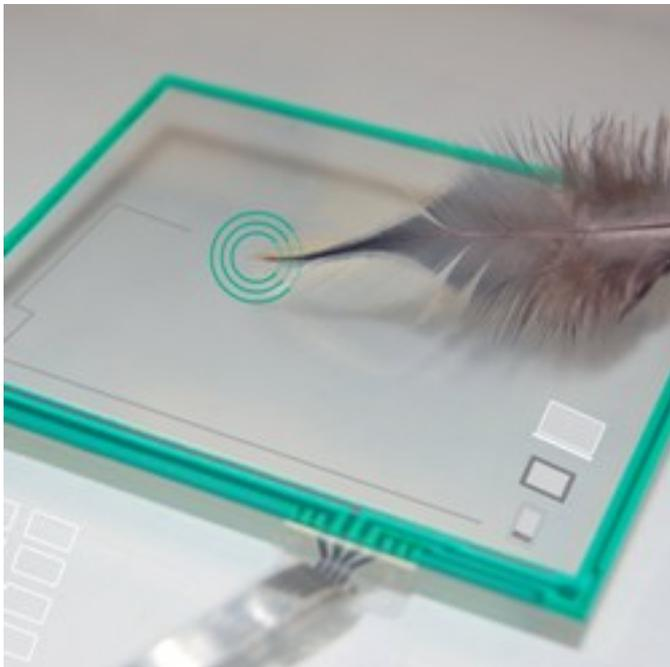
Fujitsu Components America has released a series of dual-touch, 4-wire resistive touch panels optimized for multi-touch functionality. The new panels combine the competitive features of Resistive and Projected Capacitive technology, allowing designers to expand multi-touch functionality into other applications, such as industrial equipment and controls, medical devices and automotive, using 4-wire simplicity.
