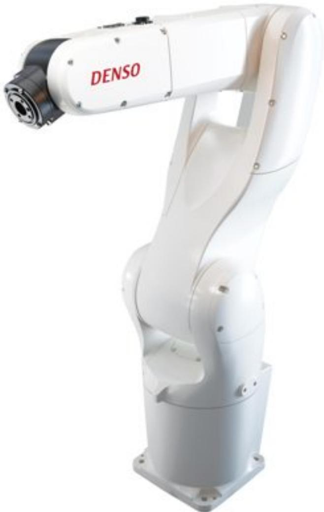
DENSO announced new ISO 3 (class 1) cleanroom versions of its VS-Series six-axis articulated robots, adding to its previously released ISO 5 (class 100) versions. The VS-Series robots offer the world's highest speed and precision in their class, with cycle times from 0.37 to 0.33 sec. and repeatability from  $\pm 0.03$  to  $\pm 0.02$  mm. Reaches are from 500 to 900 mm and payload capacities from 4 to 7 kg.
